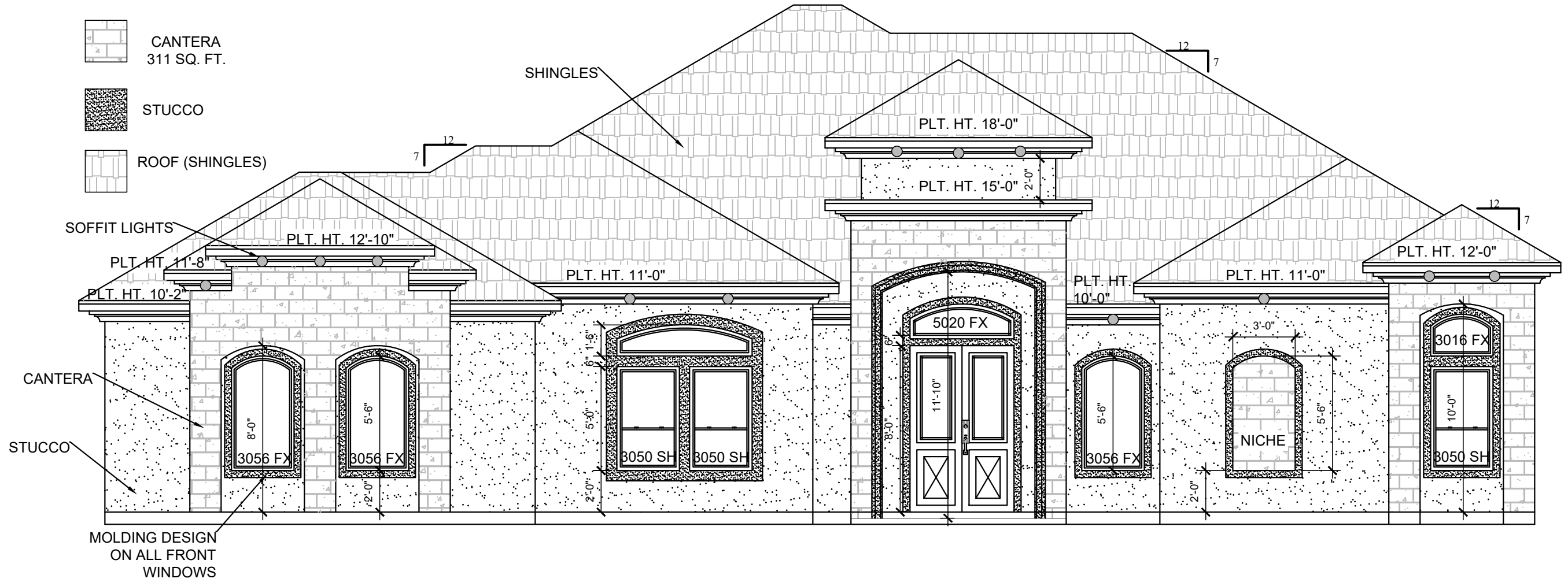
① FRONT ELEVATION SCALE: 3/16"=1'-0"
